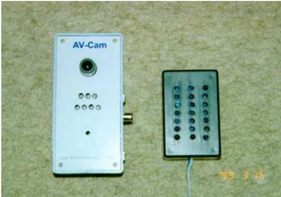
The camera within the unit is compact, approximately 2 cm in diameter and is easily focused by rotating the lens. Focal length ranges from infinity down to approximately 5 cm. The unit including the infra-red LEDs is built into a sturdy case including a microphone, video out, audio out, RF out to allow the unit to be attached directly to a monitor and power supply jacks. Additional to the camera itself are video and power supply cables which are needed to record footage onto video tape.
